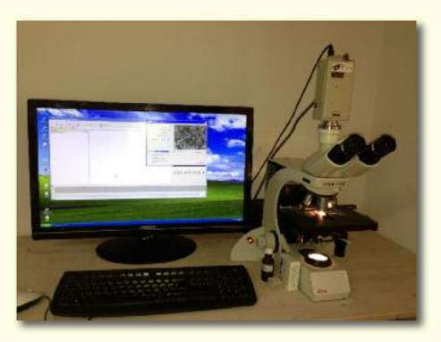
Fig. 11: Experimental setup with dark field microscope Leica DMLB
